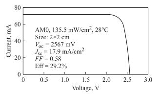
**Figure 2.** AM0 I-V curve of InGaP/InGaAs/Ge 3-junction solar cell.
