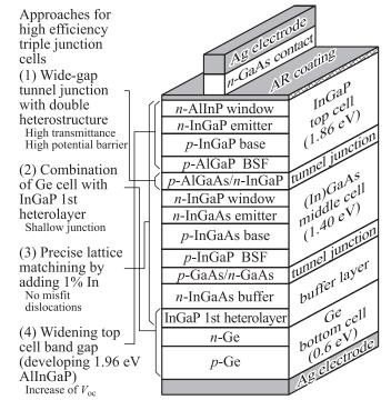
**Figure 1.** Schematic illustration of a triple-junction cell and approaches for improving efficiency of the cell. BSF — back surface field.
