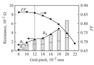
**Figure 3.** *FF* of the concentrator cells with various grid pitching under 250-sun light. Series resistance ( $R_S$ ), lateral resistance ( $R_L$ ) and total electrodes resistance ( $R_E$ ) are also shown.
