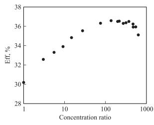
**Figure 4.** Efficiency of an InGaP/InGaAs/Ge concentrator 3-junction cell as a function of concentration ratio.
