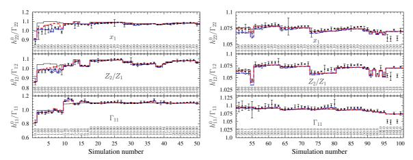
**Fig. 1** Histogram of the enhancement factors extracted from: 1) Widom fitting (dots with error bars); 2) linear mixing [Eq. (3); solid line]; 3) thermodynamics (long-dash lines); 4) our approximation [Eq. (4); short-dash lines]. (Online colour: www.cppjournal.org)
