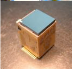
32 CdTe detectors, 1 cm 2 detector area → energy range 4 – 150 keV, resolution 1-15 keV
