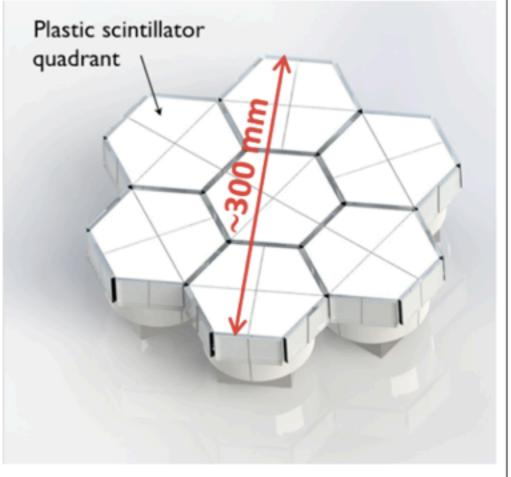
Figure 1: Overview of the SPHiNX detector. Avalanche photodiodes for reading out the BGO scintillators are not shown.
